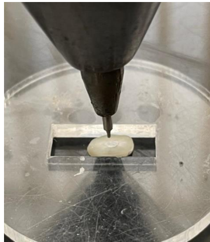
Figure 1. Push out bond strength test on the samples
