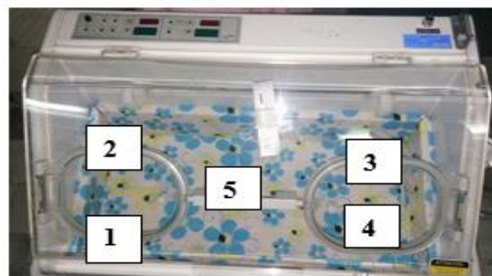
Figure 1. The points used inside the incubator to measure the magnetic field intensity
