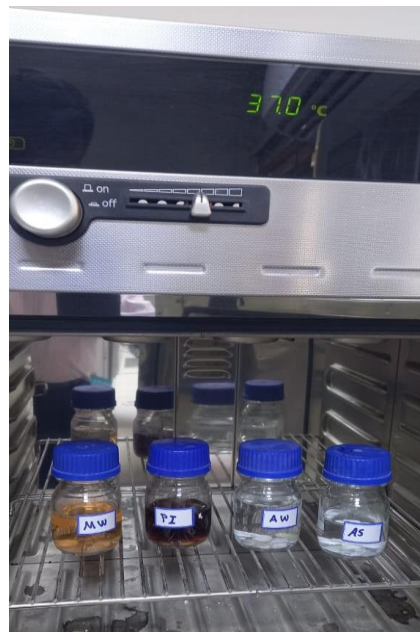
Figure 1. Shows storage of samples in solution at 37°C
