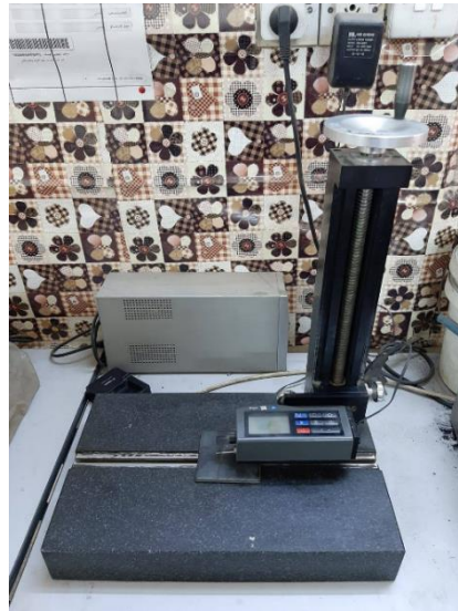
Figure 5. Profilometer (TR200, USA)
