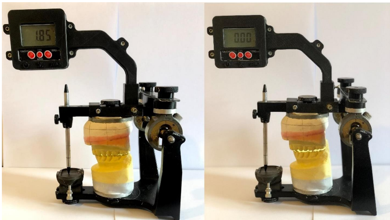
Figure 3. Articulator's upper arm inclination change following maxillary unit superior repositioning measured by the digital inclinometer
